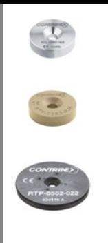
Designed for environments up to 180 or 250°C, HIGH TEMPERATURE tags offer exceptional longevity and a thermal cycling reliability of 1000 hours (or 1000 cycles). Tags are insensitive to dirt and provide between 128 and 2048 Bytes of user memory. As passive devices, no battery or other power source is required. Housings are impervious (IP 68 & IP 69K).
