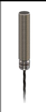
Exceptional working conditions demand uncompromising performance, and Contrinex HIGH TEMPERATURE sensors deliver in sizes M8 to M50. Designed for continuous operation at temperatures up to 180°C (up to 230°C with remote electronics), these sensors are ideal for the harshest environments, including automotive paint shops, metal-treatment plants and glass manufacturing, combining high accuracy with world-class reliability.
